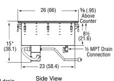
\*Manifold drain adds 6½ (16.5) to overall height
