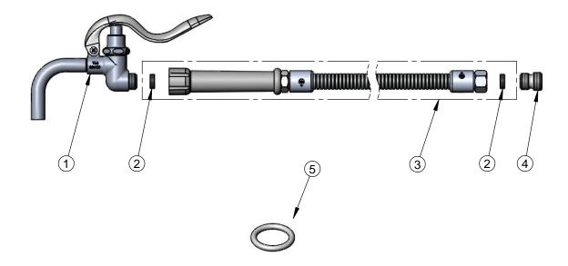
Spray Valve w/ 90° Plain End Outlet & 68" Flexible Stainless Steel Hose w/ Adapter
