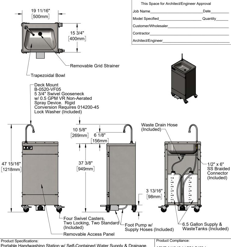
Portable Handwashing Station w/ Self-Contained Water Supply & Drainage, Deck Mount Swivel/Rigid Dummy Gooseneck w/ 0.5 GPM Vandal Resistant Non-Aerated Spray Device, Swivel Casters and Foot Pump
