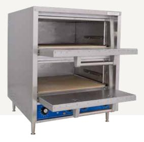
Bakers Pride® P48 series ovens feature two independently controlled baking chambers, each with one deck in your choice of Cordierite (7" height) or bricklined Cordierite (7.5" height). The greater deck height allows you to accommodate taller bake and roast items. The brick-lined model adds a Cordierite ceiling, which offers the benefit of increased temperature and recovery time. They may be easily installed at the factory or in the field.
