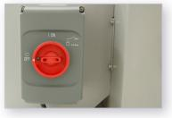
To switch machine on, turn the knob rotation clockwise to the on position. To switch the machine off, turn the knob rotation counterclockwise towards the off position.
