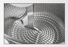
Both bowl and spiral are made from high-resistance stainless steel.
