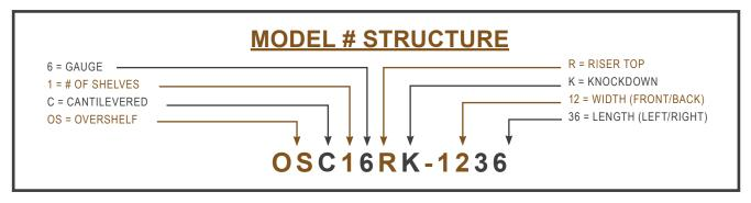
SOME UNITS SHIP UNASSEMBLED FOR REDUCED SHIPPING COST. ALL DIMENSIONS ARE TYPICAL. TOLERANCE +/- .500" John Boos & Co. is constantly engaged in a program of improving products and therefore reserves the right to change specifications without prior notice.
