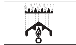
BURNER HEATS RADIANT WHICH RADIATES HEAT TO THE GRATE AND FOOD ITEM.
