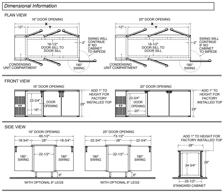
Note: Available with compressor left or right. Compressor left model shown.
