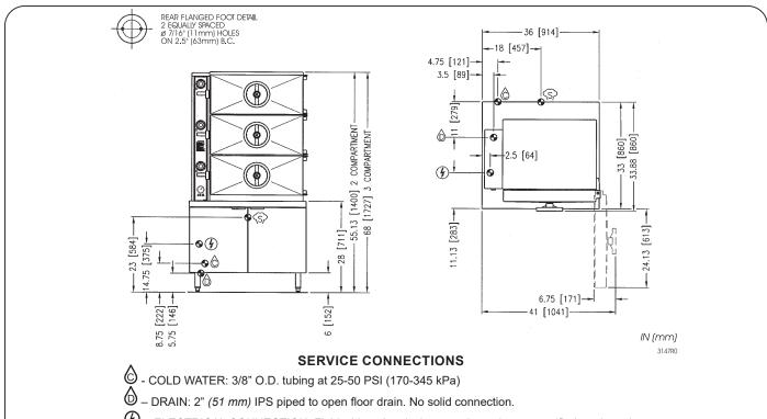
⑦ – ELECTRICAL CONNECTION: Field wiring electrical connection to be as specified on data plate.
