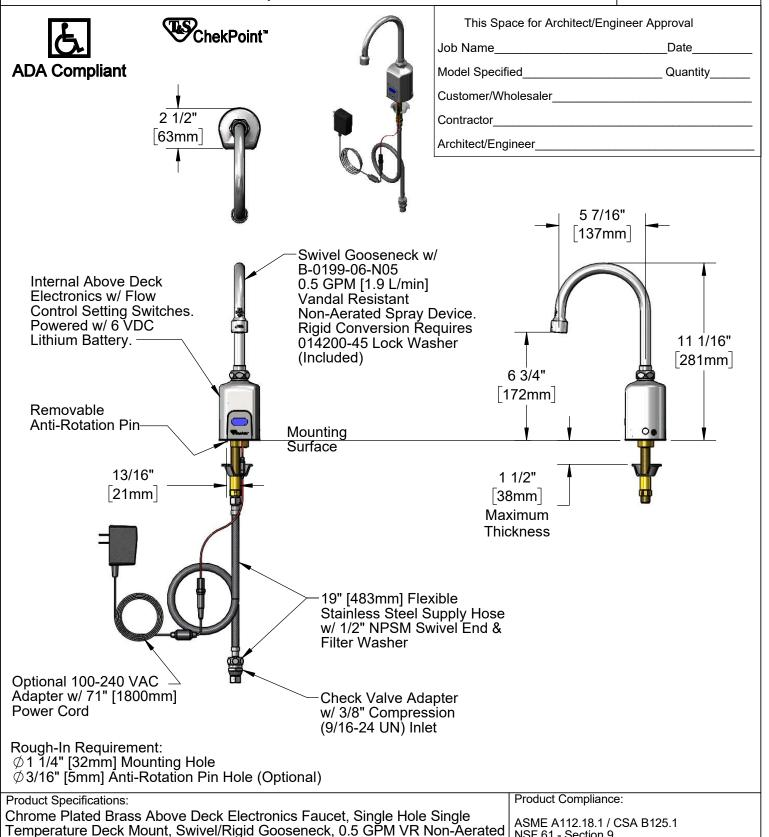
Spray Device, Battery or AC Adapter Powered, 19" Flexible Stainless Steel
