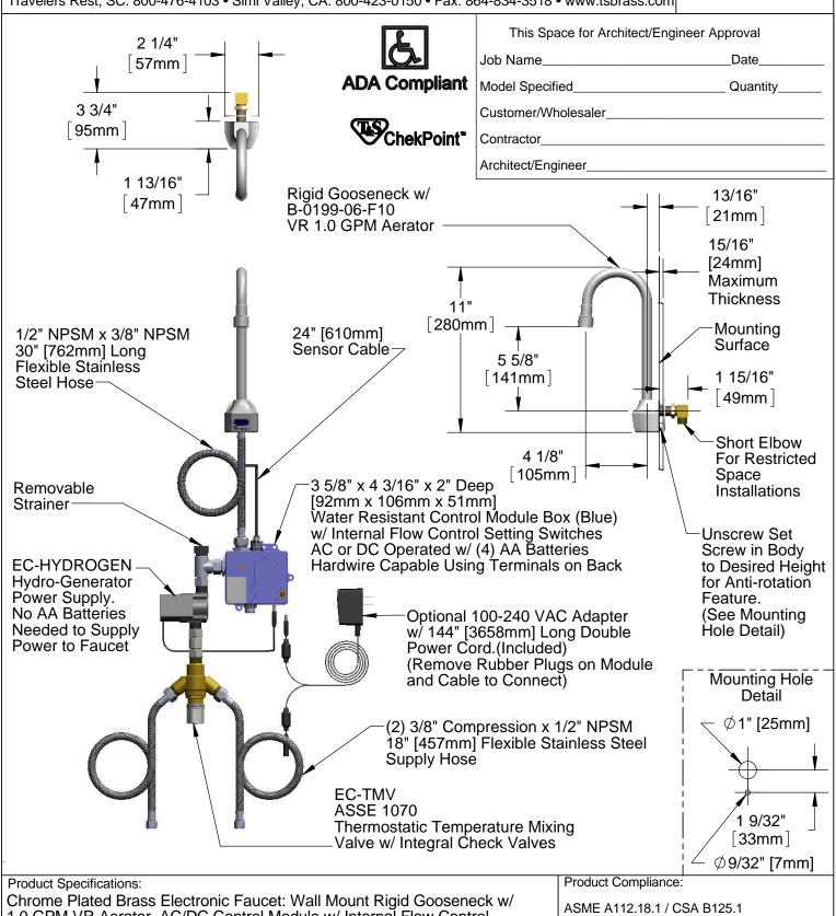
1.0 GPM VR Aerator, AC/DC Control Module w/ Internal Flow Control Setting Switches, Thermostatic Temperature Control Mixing Valve w/ Integral Check Valves, Hydro-Generator, 18" Hot & Cold Flexible Connector Hoses
