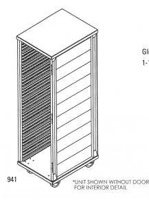
Glides are channels spaced on 1-1/2" centers with 5/8" ledge
