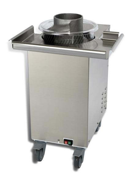
Automatic Dough Rounder, Rounds Up to 800 Portions per Hour, Rounds Portions Ranging from 7-36 Oz, Recommended for Doughs with 60% Hydration or Higher, 6" Entry Chute, Stainless Steel Construction, 120V/60/1P/6A, NEMA L5-15P, cETLus, ETL-Sanitation
