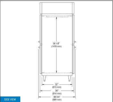
**IMPORTANT NOTE:** If the cabinet is located under a low ceiling, a <u>minimum</u> <u>clearance of 12" is required on top and 3" on sides.</u>
