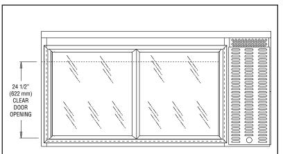
**IMPORTANT NOTE:** Models are completely front breathing and take in and exhaust air through the front grill. For proper operation, the area in front and back of the cabinet must not be obstructed in any way. A clearance of 3" on the sides is recommended.
