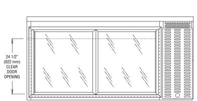
**IMPORTANT NOTE**: Models are completely front breathing and take in and exhaust air through the front grill. For proper operation, the area in front and back of the cabinet <u>must</u> not be obstructed in any way. A clearance of 3" on the sides is recommended.
