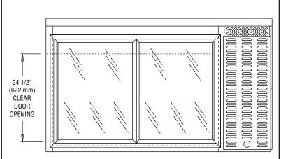
**IMPORTANT NOTE:** Models are completely front breathing and take in and exhaust air through the front grill. For proper operation, the area in front and back of the cabinet **must** not be obstructed in any way. A clearance of 3" on the sides is recommended.
