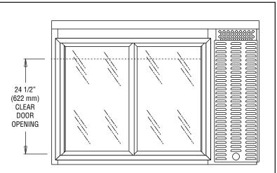
**IMPORTANT NOTE**: Models are completely front breathing and take in and exhaust air through the front grill. For proper operation, the area in front and back of the cabinet <u>must</u> not be obstructed in any way. A clearance of 3" on the sides is recommended.
