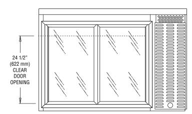
$\underline{\textbf{IMPORTANT NOTE}}\text{: Models are completely front breathing and take in and exhaust air through the front}$ grill. For proper operation, the area in front and back of the cabinet must not be obstructed in any way. A clearance of 3" on the sides is recommended.
