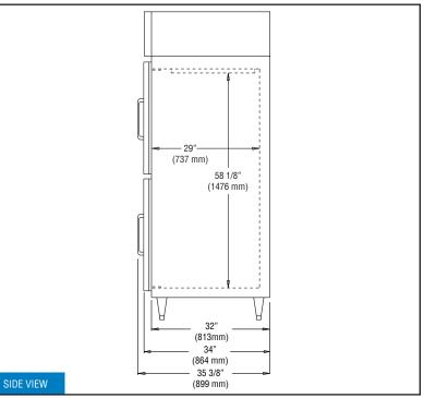
**IMPORTANT NOTE**: If the cabinet is located directly against a wall and/or under a low ceiling, a <u>minimum</u> clearance of 12" is required on top and 3" on sides and rear.
