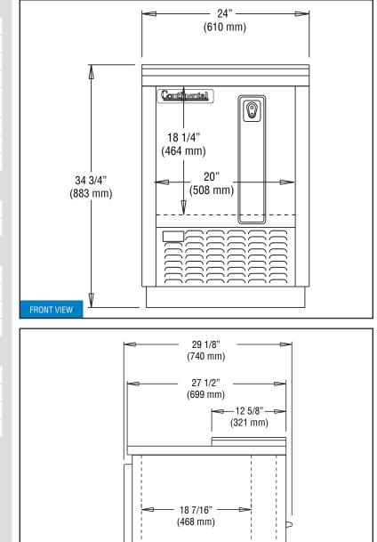
**IMPORTANT NOTE**: Model is completely front breathing and takes in and exhausts air through the front grill. A clearance of 1" on the back and 3" on the sides is recommended.
