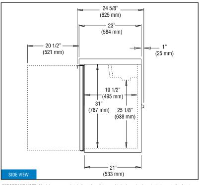
**IMPORTANT NOTE**: Models are completely front breathing and take in and exhaust air through the front grill. For proper operation, the area in front of the cabinet <u>must</u> not be obstructed in any way. A clearance of 1" on the back and 3" on the sides is recommended.
