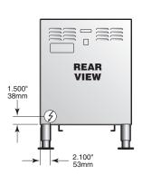
**ELECTRICAL** (Contact factory if installed above 3,500 feet)
