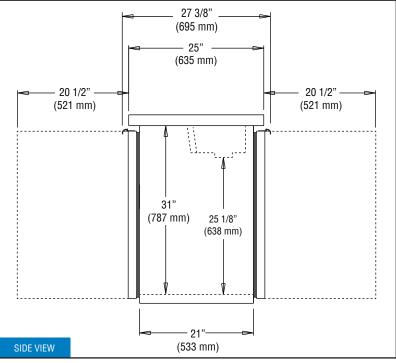
**IMPORTANT NOTE**: Models are completely front breathing and take in and exhaust air through the front grill. For proper operation, the area in front of the cabinet <u>must</u> not be obstructed in any way. A clearance of 3" on the sides is recommended.
