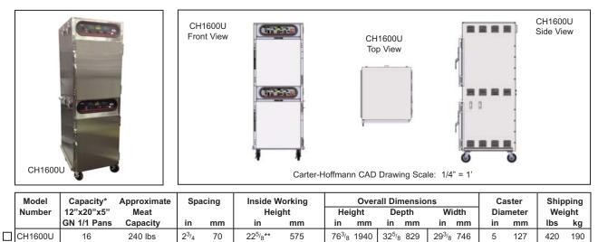
\*CH1600U accommodates (16) 12"x20"x2.5" and GN1/1 pans, side-loaded (2 per shelf), or (8) GN2/1 pans per cavity; will accommodate (8) 18"x26", end-loaded, on optional wire shelves, per cavity.
