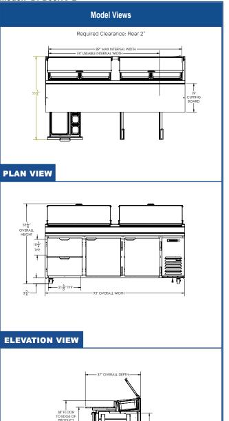
\*NOTE: Remote units are field wired and come with 6" legs. Refrigerant must be specified at time of order.
