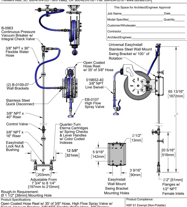
Open Coated Hose Reel w/ 35' of 3/8" Hose, High Flow Spray Valve w/ Swivel, Vacuum Breaker, 3/8" NPT Flexible Water Hose, 100 Degree EasyInstall Stainless Steel Swing Bracket, 8" Deck Mount Mixing Faucet w/ Spring Checks, (2) Wall Brackets & Control Valve
