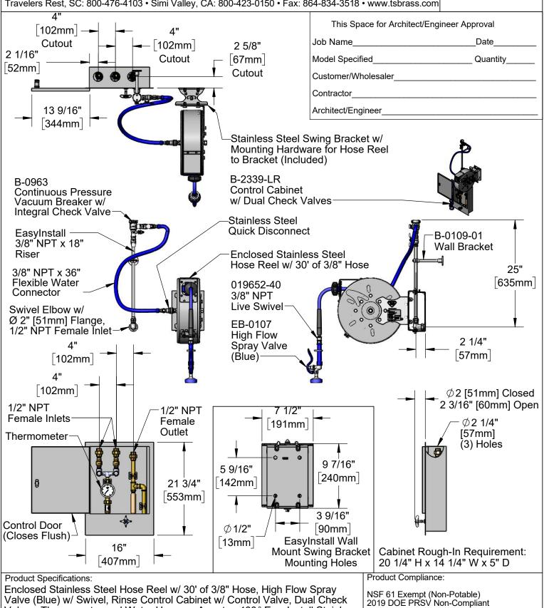
Valves, Thermometer and Water Hammer Arrestor, 100° EasyInstall Stainless Steel Swing Bracket w/ Mounting Hardware for Hose Reel to Bracket & Hose Reel Connector Kit
