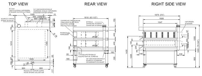
Note: The dimensions indicated in the views are in millimeters. Steamer for Bakery only.
