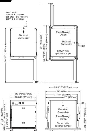
**Dimensions:** H x W x D **Exterior:** 31-7/8" x 26-5/8" x 31-5/8" (809mm x 676mm x 802mm)
